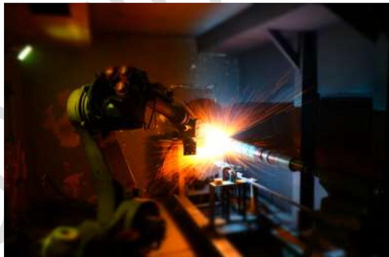
*Figure 2: Arc Wire Spraying*
